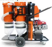
The three separate filtering stages result in longer working time between filter cleaning. The dust is filtered through a cyclone chamber, which separate the heaviest parts, up to 95% of the dust, before the washable main filter. The HEPA micro filters are individual tested and certified to capture 99.99% of the remaining silica dust in the respirable fraction (0.3µm).
