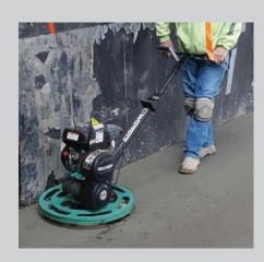
Allows finishing within 7/16" of any obstruction
